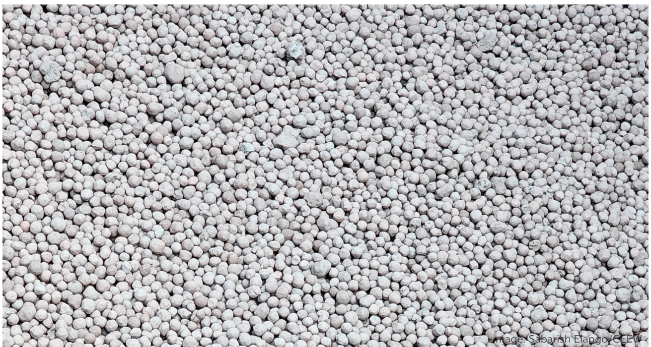
Spherical iron ore pellets are used in the DRI kiln when higher-grade lump ore is not available.
