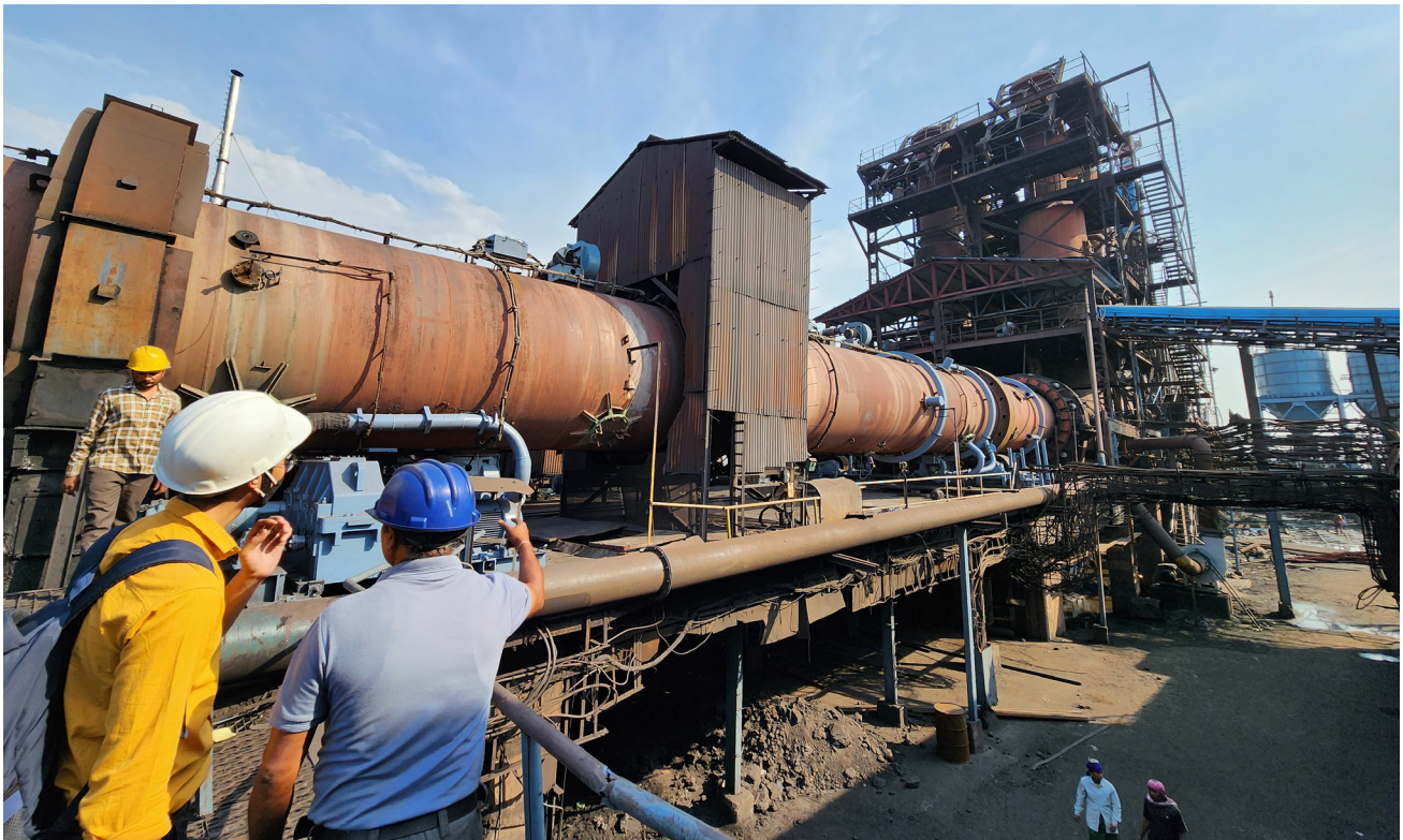
CEEW's researchers visited a 200 tonnes per day (TPD) coal-DRI rotary kiln in Raipur, Chhattisgarh, as part of the DRI plants survey.
