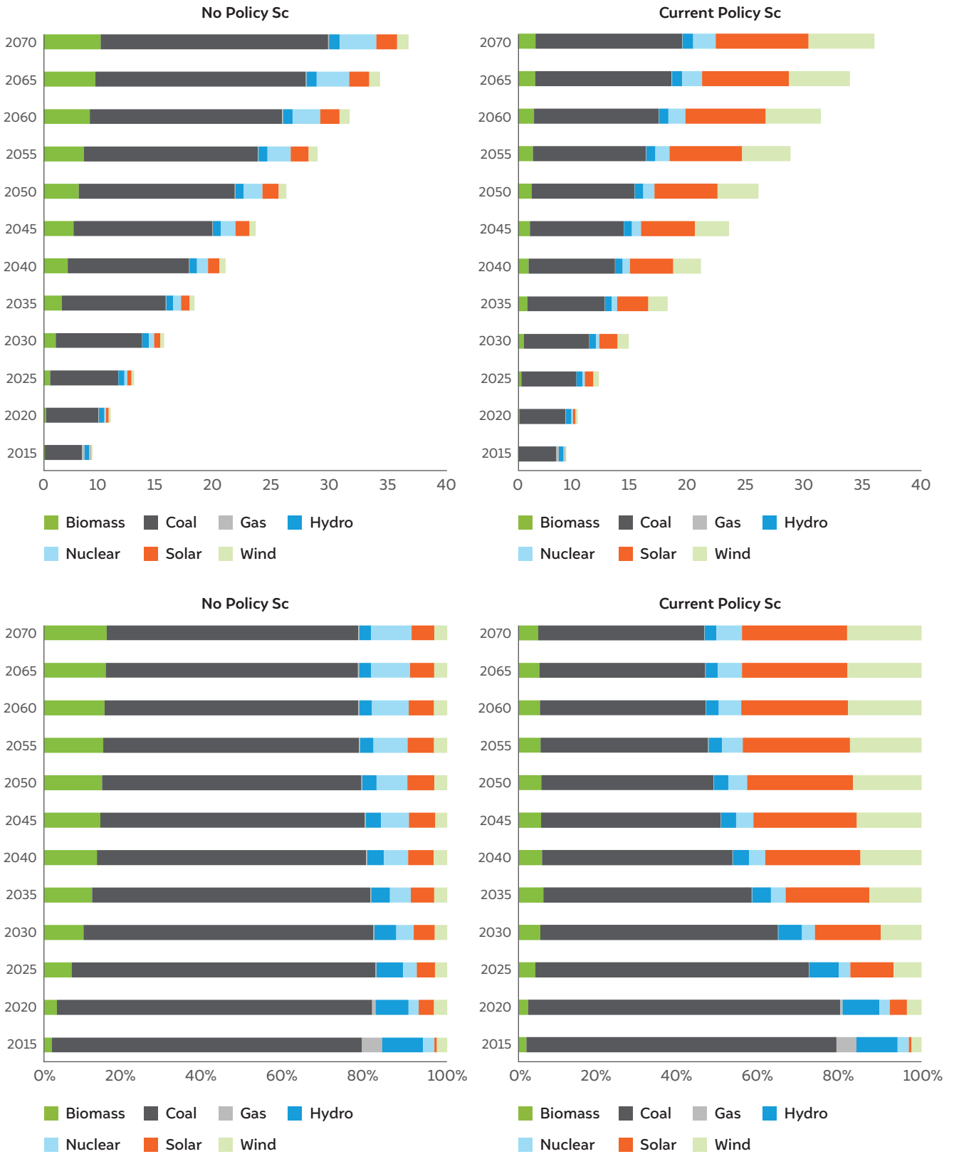
Figure 2 (a) Electricity generation mix by fuel (Exa-Joules [EJ]) (b) Electricity generation shares by fuel (%)
