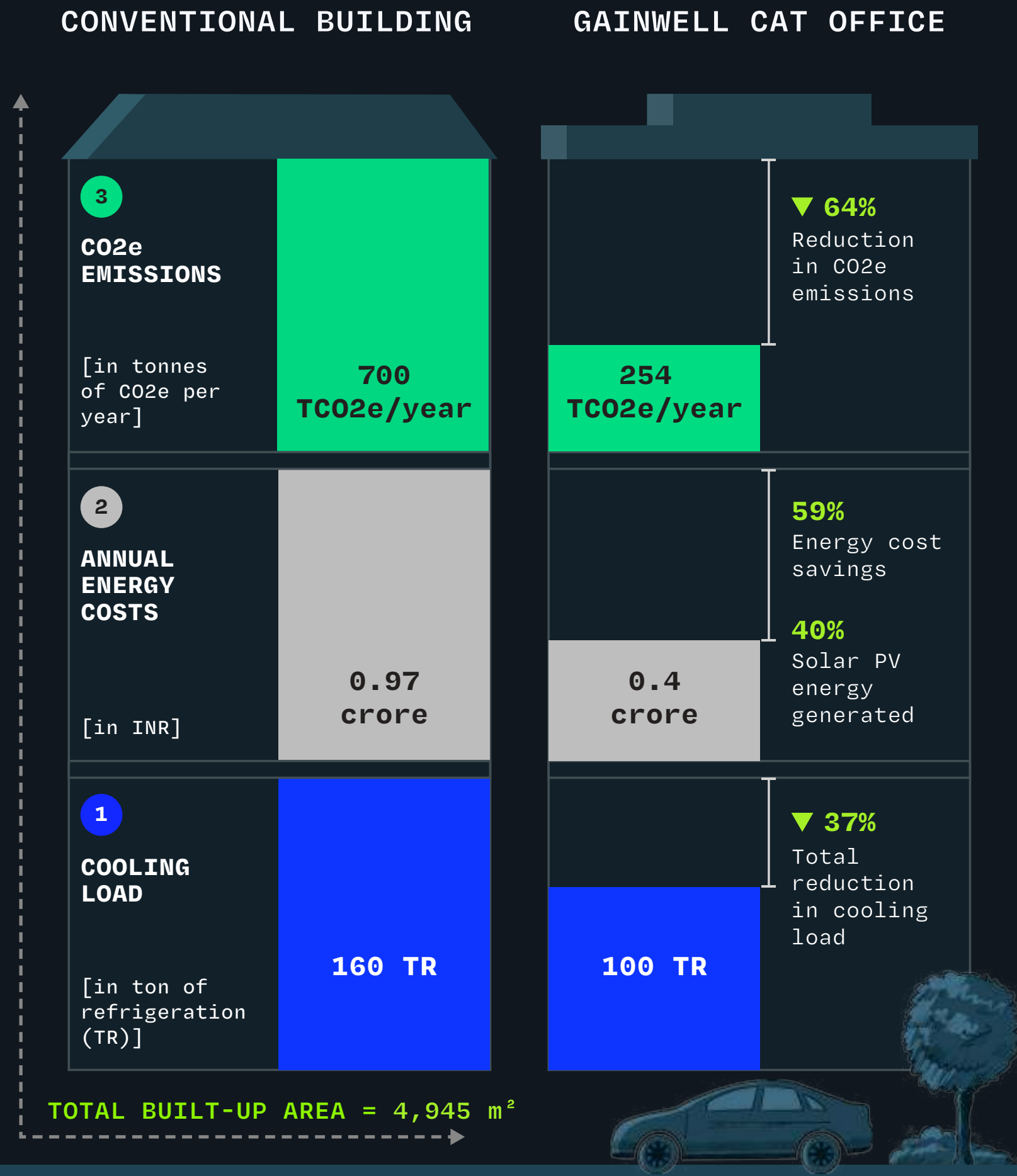
EXHIBIT 41: Energy performance of Gainwell CAT office building
